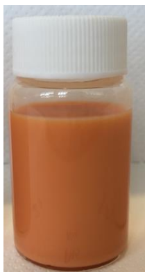
Figure 6.3- Astaxanthin-loaded NLCs: Produced using a formulation without organic solvent through melt-emulsification using a homogenization time of 20 minutes and speed of 21500 rpm.
