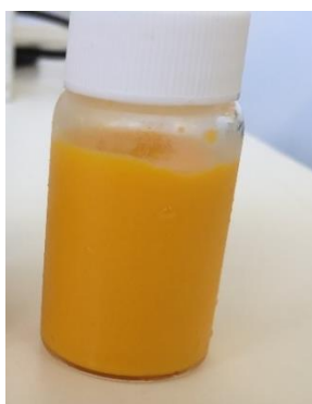
Figure 6.2- \beta -carotene-loaded NLCs: Produced using a formulation without organic solvent through melt-emulsification using a homogenization time of 7 minutes and speed of 21500 rpm.
