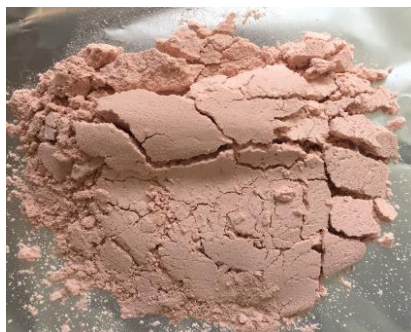
Figure 3.5- Astaxanthin-loaded SLCs produced using a formulation containing olive oil, through PGSS® precipitation at 70°C, 250bar and 15 minutes as contact time with scCO 2 .
