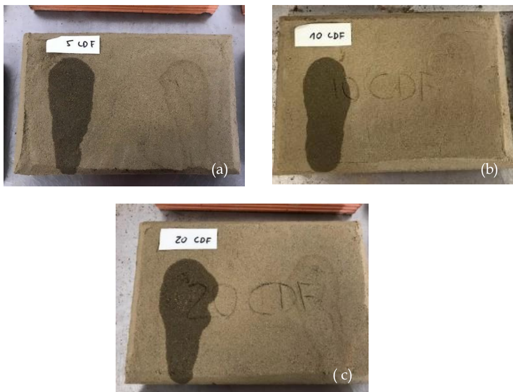
Figura 4.15. Área erodidas dos rebocos CAP(1:1,5)+5EBfp7(AF) (a), CAP(1:1,5)+10EBfp7(AF) (b) e CAP(1:1,5)+20EBfp7(AF) (c)
