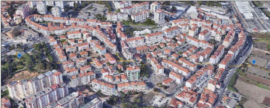
Figure 5.2: Satellite image of the test site location in Povoia de Santo Adrião with a yellow line between the base station and the module. The module is on the left side, the base station is on the right, and the distance between them is 530 meters.
