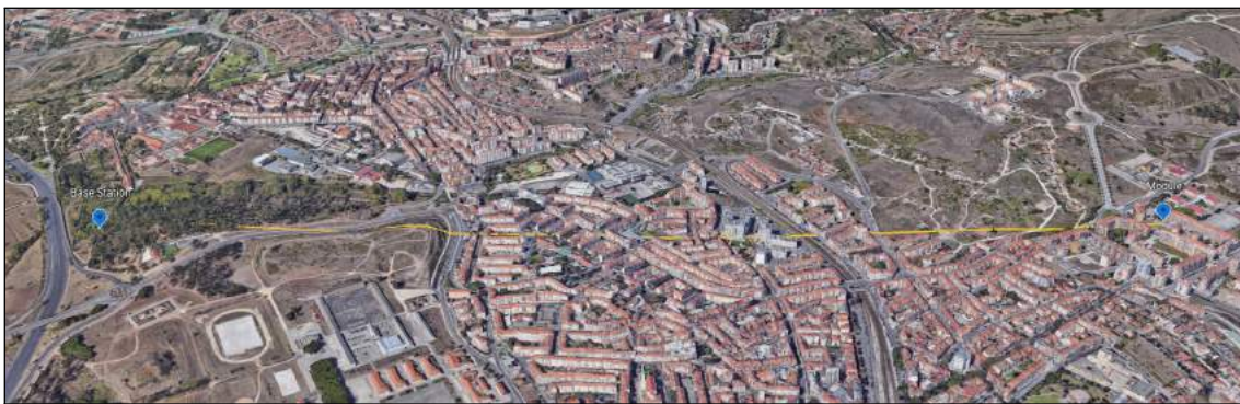
Figure 5.3: Satellite image of the test site location in Vila Chã with a yellow line between the base station and the module. The module is on the right side, the base station is on the left, and the distance between them is 2260 meters.
