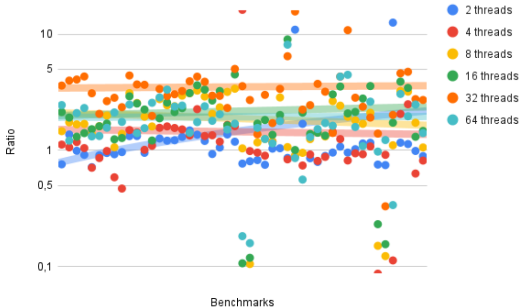
Figure 4.10: Ratio of unsuccessful steals of WShare using tit-for-tat heuristic over LCWS on machine AMD 32-64.
