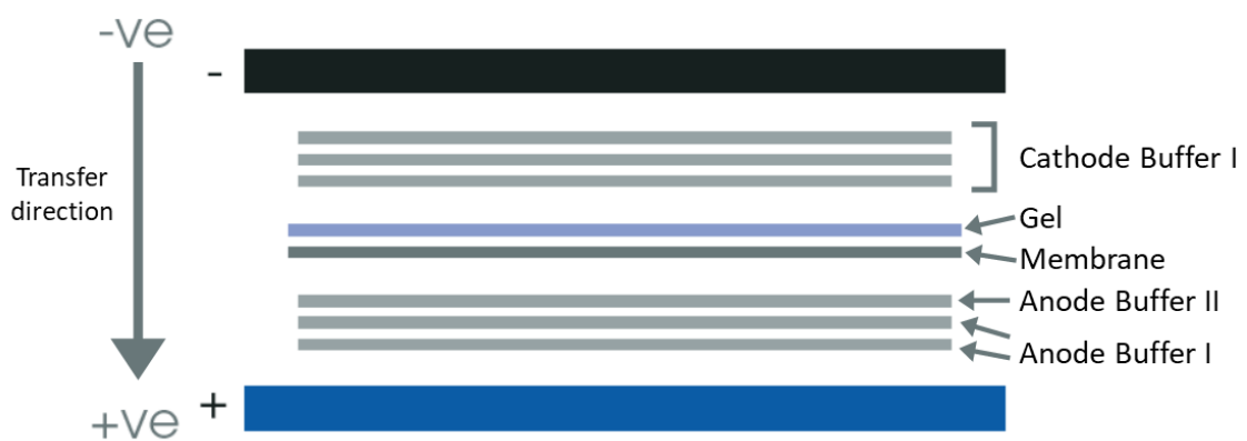
Figure A6- Semi-dry transfer system representation. Adapted from Abcam's General western protocol.
