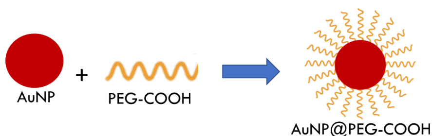
Figure 2.1- Representation of citrate capped gold nanoparticle (AuNP) functionalization with polyethylene glycol harboring a carboxylic acid functional group (SH-EG(8)-COOH) (PEG-COOH).
