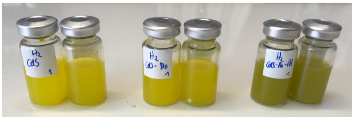
Figure 3.1: Example of photocatalytic flasks containing duplicates of different Desulfovibrio -biohybrid systems for light-driven H_2 production assays
