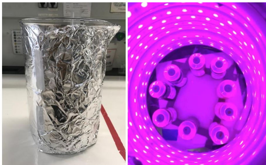
Figure 3.3: Photocatalytic flasks in experimental setup arranged within 5 L glass beaker (right) under violet LED irradiation (left)
