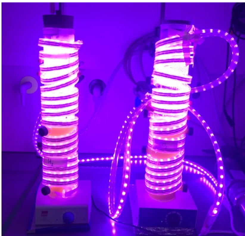
Figure 3.2: Bench-scale reactors for the light-driven production of H 2 (left) and the light-driven reduction of CO 2 (right)
