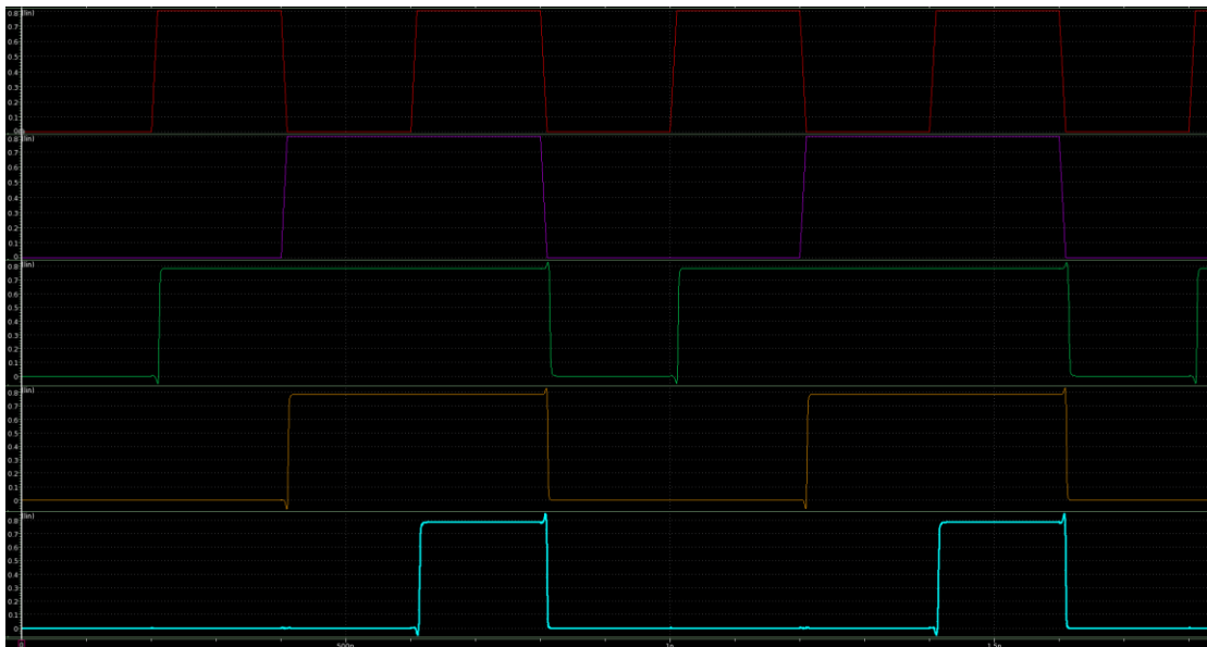
Figure 73: Output voltages of the decoder for signals t0 (green), t4 (orange) and t8 (blue).
