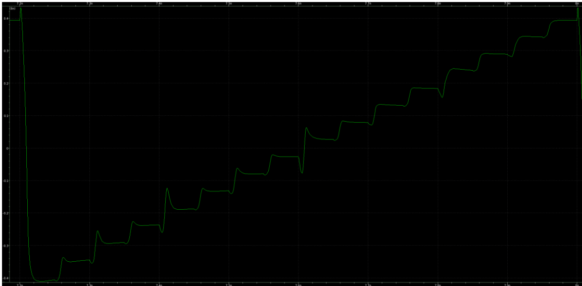
Figure 53: DAC response for 10GHz sampling.
