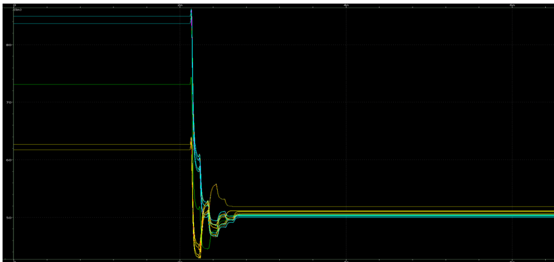
Figure 63: Output impedance during calibration for 65 corners.
