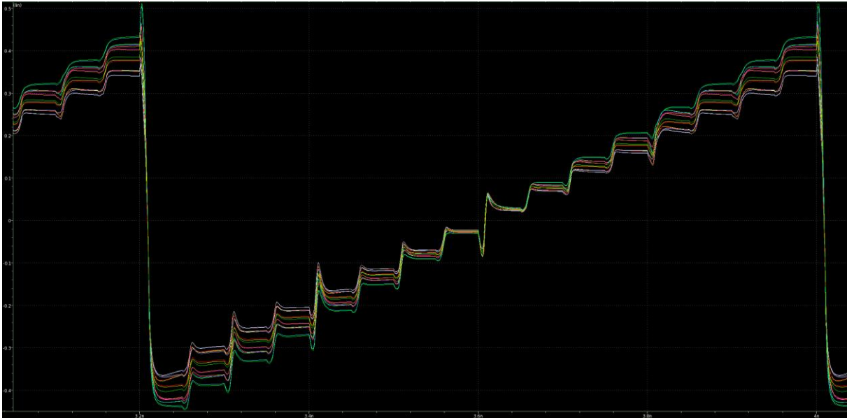
Figure 58: DAC response for 10GHz sampling and 17 corners.
