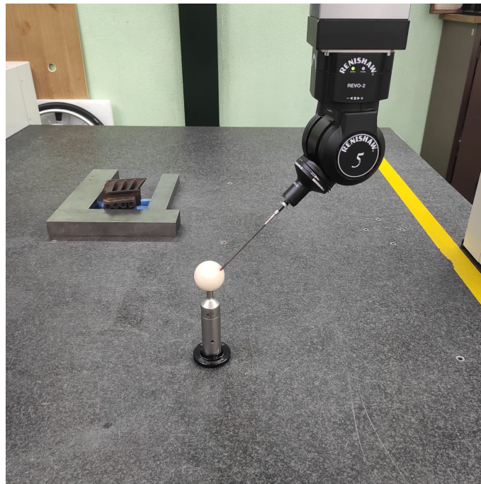
Figure 7.8: Calibration to position \beta = 75^\circ and \theta = 45^\circ .
