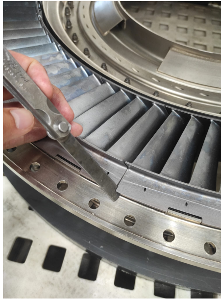
Figure 6.9: Method to measure clearance between nozzles segments.
