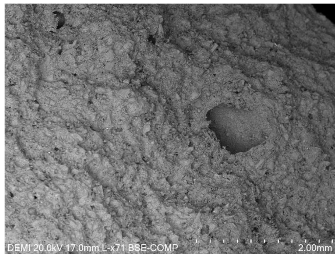
Figure 3.20 SEM image of 19,5 %(V/V) SiC sample's fracture site.
