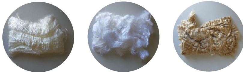
Figure 4.1 - Samples of the fibres in study (from left to right: raw white, dyed and pigmented).
