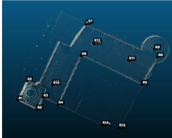
Fig. 14 Manual alignment between reconstructed model and LiDAR reference.
