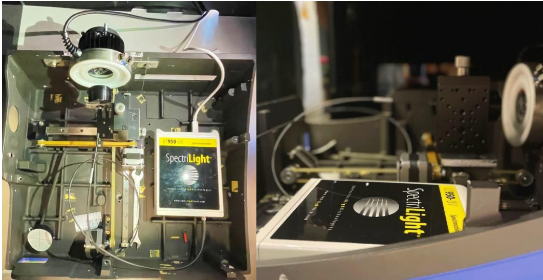
Figure 3 - Setup used for the measurement of the light intensity of the LEDs that emit light at different wavelengths.
