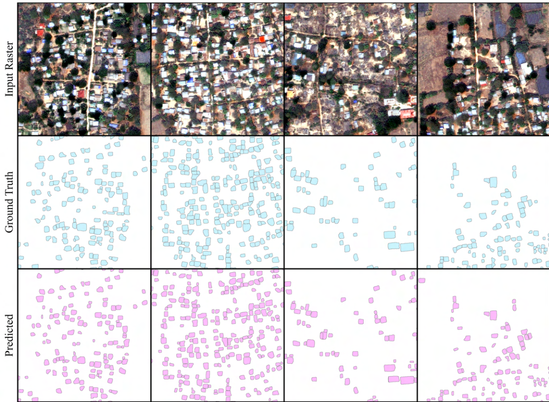
Figure 18: Input images and building polygons extracted by trained Mask R-CNN model visualized against ground truth polygons.
