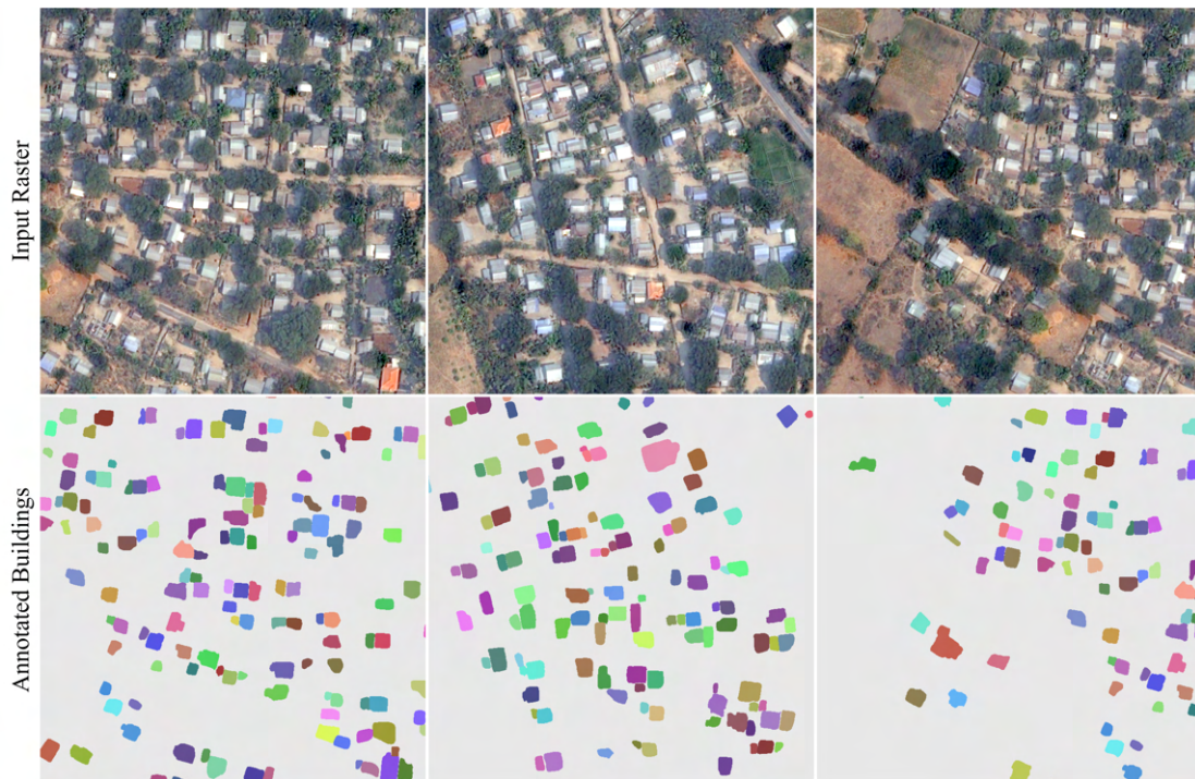
Figure 15: Input RGB raster tiles and building annotations used in the training process of Mask R-CNN model.
