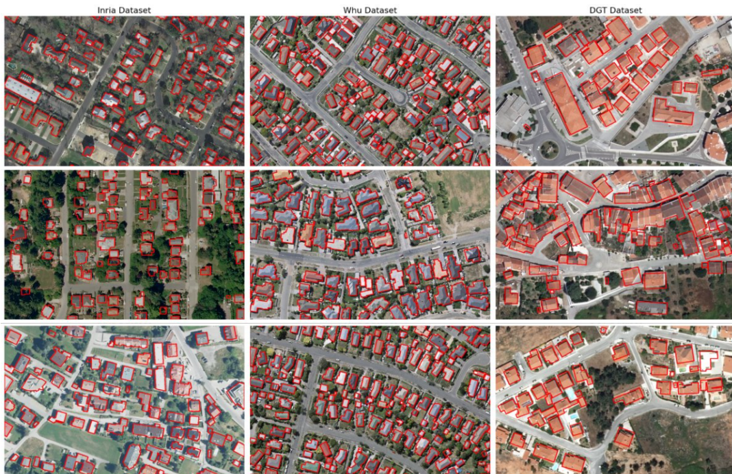
Figure 4.3: Annotations derived from the Inria Aerial Image Labeling dataset, the Whu Aerial Building dataset and the DGT Real Color Dataset.
