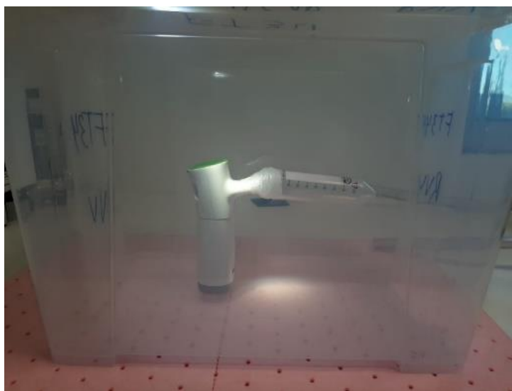
Figure 8 Nebulization set up, inside a closed box to contain the release of droplets to the surrounding environment, due to HSE concerns.
