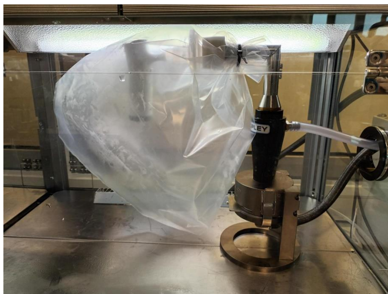
Figure 10 Delivered Dose set up for nebulized solutions using a jet nebulizer inside a plastic bag due to health, safety, and Environment (HSE) concerns [123].
