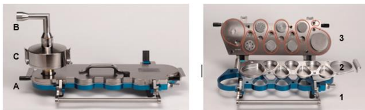
Figure 4 Next generation impactor left: A- 7-Stage apparatus; B- Induction Port; C- Pre-separator (does not apply to nebulizer testing) Right: 1- Bottom frame; 2- Support tray; 3- Lid with interstage
