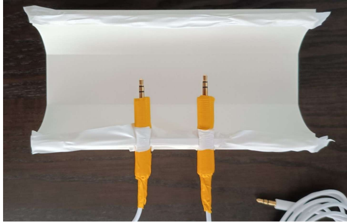
Figure 5.4: Ear-EEG phantom assembly - antennas and railing fittings are sealed with tape
