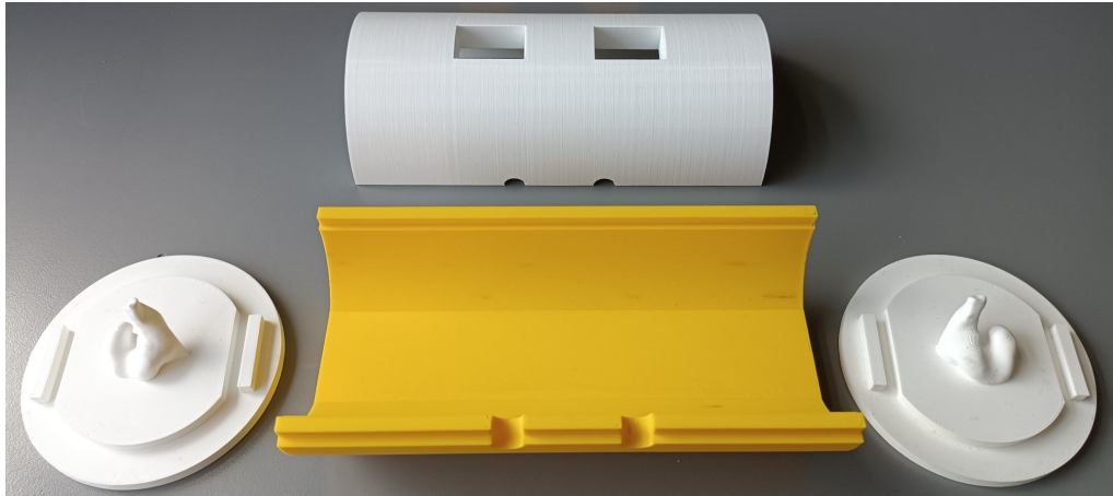
Figure F.2: Disassembled ear-EEG phantom - bottom half (in yellow), top half (in white, similar to yellow), and two lids with a left and right ear imprint from one of the subjects
