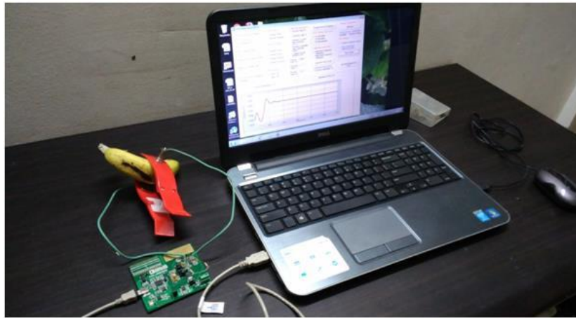
Figure 3.5 — Experimental setup using clamp electrodes (adapted from Kulkarni, 2017)
