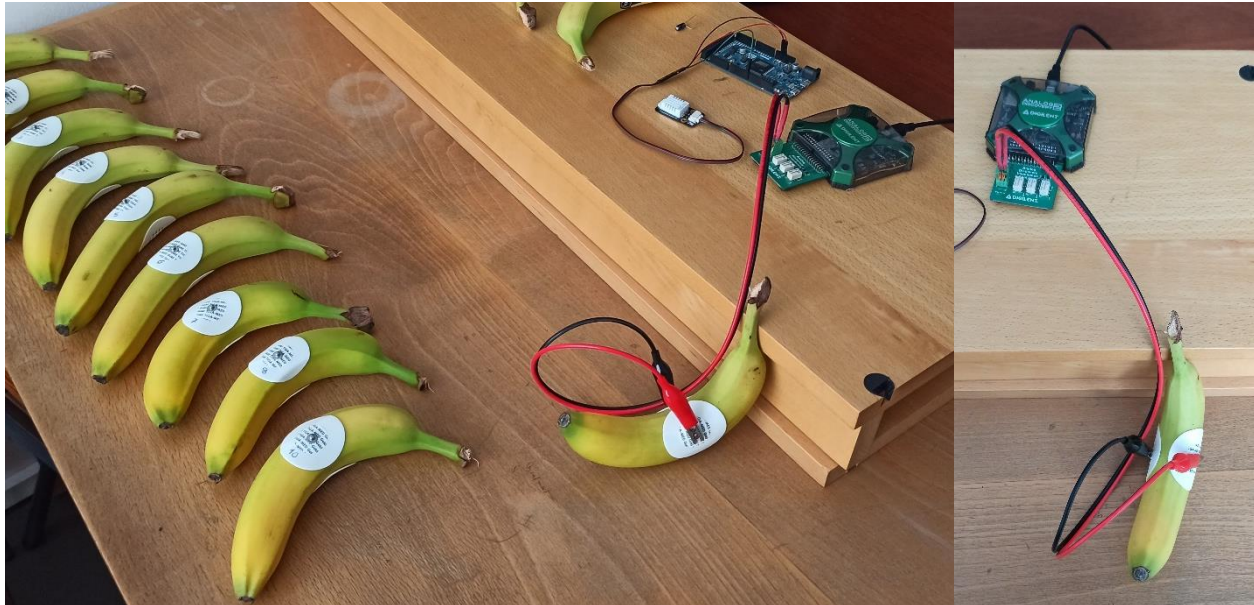
Figure 4.1 — Experimental setup, with the AD2 connected to the banana's ECG electrodes
