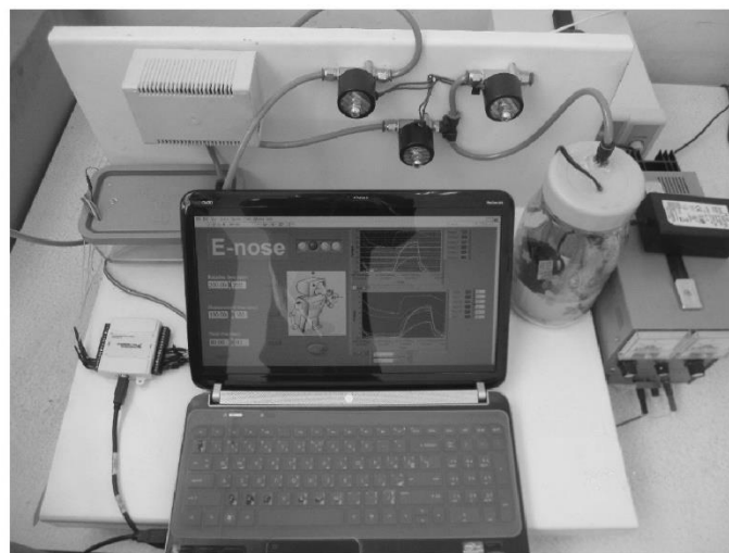
Figure 3.1 — Electric nose experiment setup (adapted from (Sanaeifar et al., 2014))
