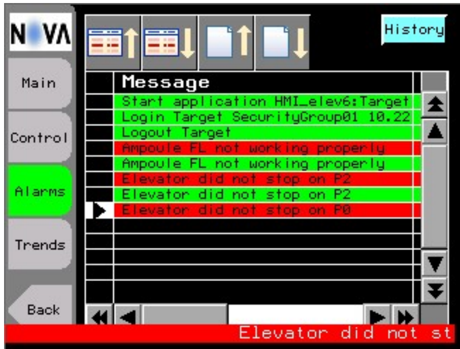
Figure 3.30: Alarm panel from the HMI.
