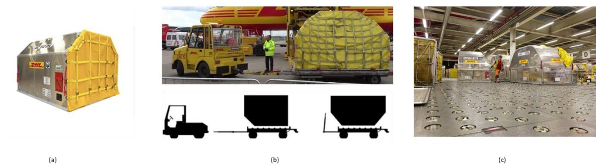
Figura 3.2: (a) ULD; (b) Dolly; (c) Castor decks
