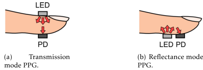
Figure 2.2: LED and photodetector (PD) placement for both modes of PPG, [24].
