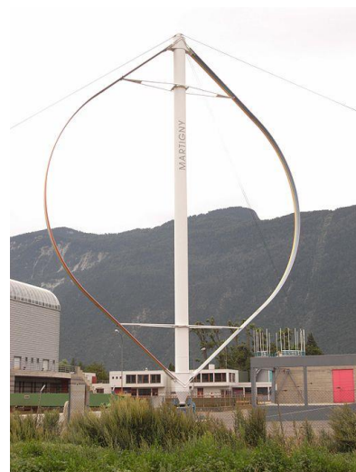
Fig. 1b: Vertical-axis wind turbines (VAWTs) Source: Lysippos, Wikimedia Common author (public domain).
