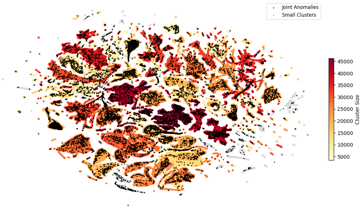
Figure 15 – UMAP Projection for the GMM and DBSCAN Anomaly Detection Model
