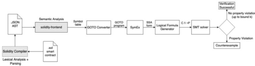
Figure 3.1: Architectural overview of ESBMC with its extension for verifying Solidity Smart Contracts. [34]
