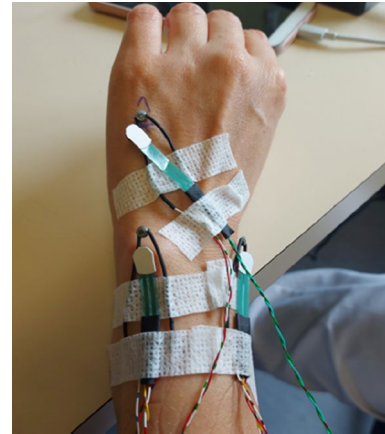
Fig. 6 Pressure and temperature sensors placed in the upper limb
