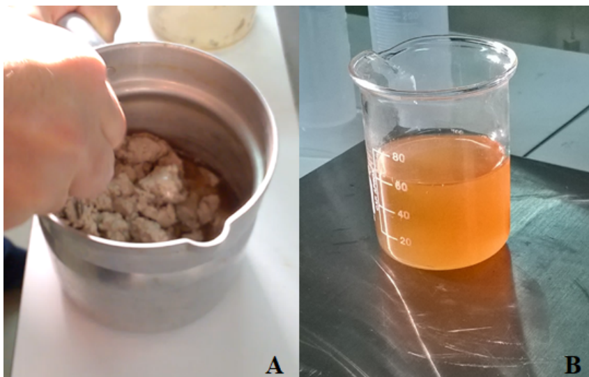
Figure 5.68: Sample taken from a mixture batch of grout material, water and microencapsulated PCM. Image A shows evidence of the heterogeneous mix unlike seen in Figure 5.67, with the PCM not staying within the designed encapsulation leeching into the water, as shown in B.
