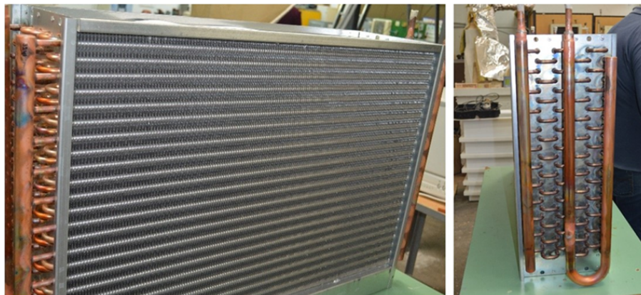
Figure 5.57: Heat exchanger full-scale prototype.(Photo courtesy of NKUA [122])
