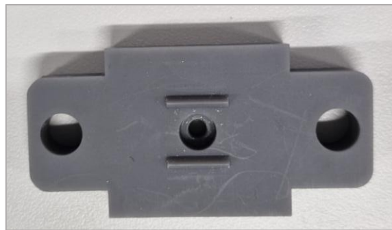
Figure 21 - 3D piece used for inner support on the four-point bending setup.
