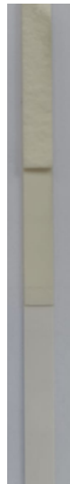
Figure 18 - Result of the 0.5pmol sample of Z 2 T with AuNPrs@Glutathione after 30 minutes of drying.
