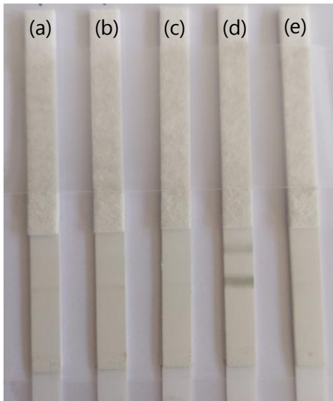
Figure 49 - Test of specificity for Z 8 T [1/1] (left) and Z 8 D [1/1] (right) for different target solution of 0.5 pmol mixed with DeltaLab matrix: (a) RSV1; (b) RSV2; (c) cc1; (d) Z 8 and (e) Z 2 .
