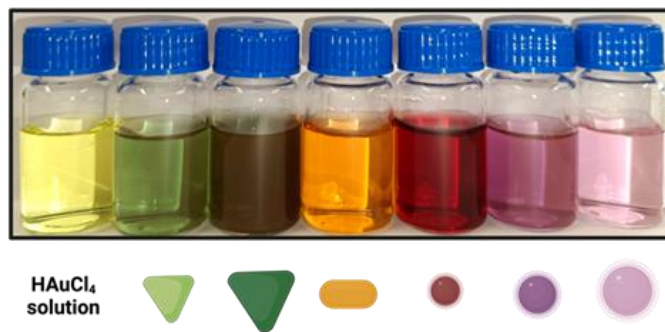
Figure 4 - Illustration of different gold nanoparticles synthesized in BioNANOSurf laboratory with different size, shape and consequently different LSPR and optical properties.
