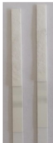
Figure 41 - Testing 0,5pmol target in DeltaLab matrix using pre-incubation of 15 minutes (right) and without pre-incubation (left).
