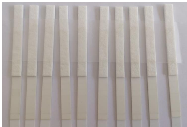
Figure 39 - Example of Z 2 T [1/16] in DeltaLab matrix, with Tris 50 mM pH 9 100 mM NaCl showing the presence of ghost effect.
