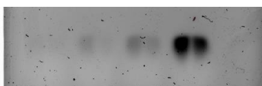
Figure 24 - Gel of biofunctionalization of AuNPrs@PEG with Z 8 D. Layout from left to right is Stock and Supernatant, where the concentrations are respectively, [1/16]; [1/8]; [1/4] and [1/1].
