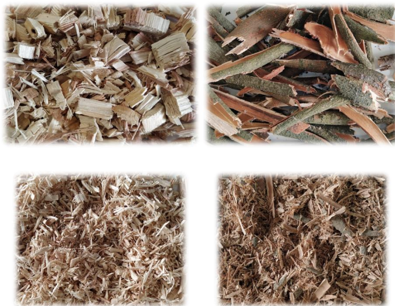
Figure 7.1 — Shredded wood (top, left) and bark (top, right); grounded wood (bottom, left) and bark (bottom, right).
