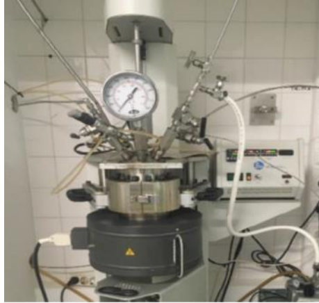
Figure 9.2 — Stainless steel autoclave reactor used in the HTC experiments.
