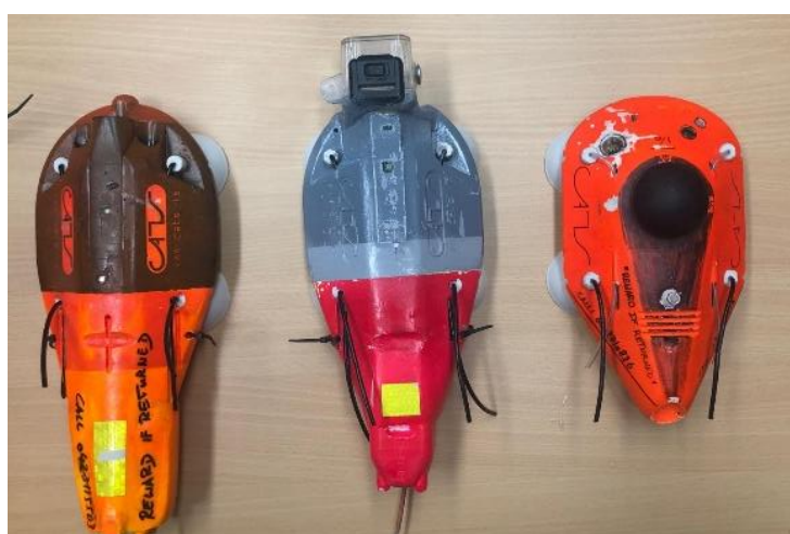
The photo shows various tags that are attached to the whale's skin using suction cups.
