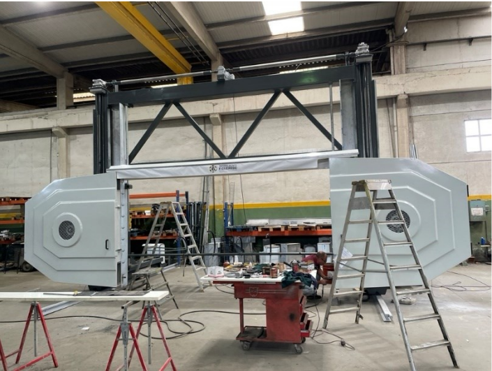
Appendix 12 One slate block cutting machine
