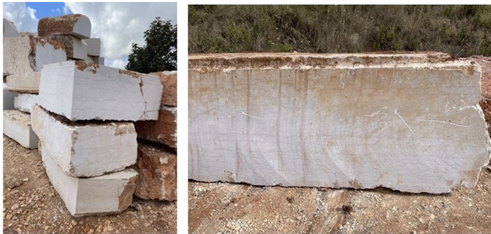
Figure 16 Examples of low-quality raw blocks, photos Nuno Castanheira
