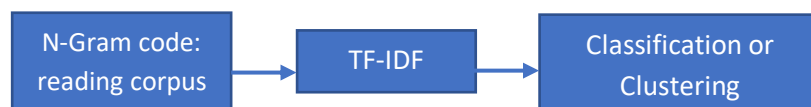
Figure 6. The n-gram pipeline when analyzing a text body using TF-IDF technique resulting in an output which is text classification or clustering of words.
