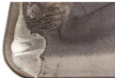
Figure 2.18: Crater wear - Example [41]
