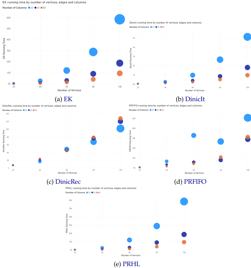
Figure 3.11: Algorithms' running times by number of vertices for random layered networks - The number of edges is coded in the circles' sizes and the color codes the number of columns.
