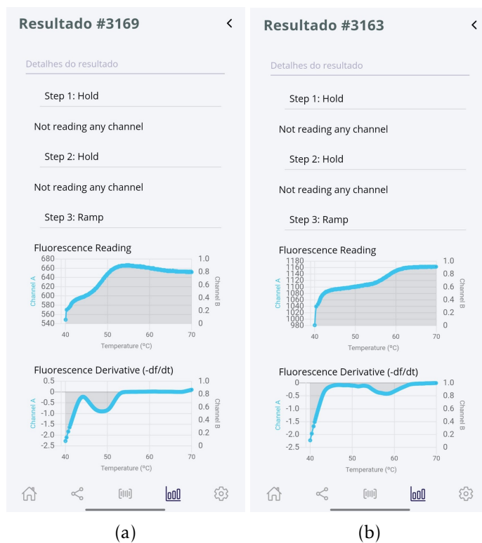
Figure 6.10: Application result page: a) Ramp analysis with a CC result made by the application, b) Ramp analysis with a TT result made by the application.
