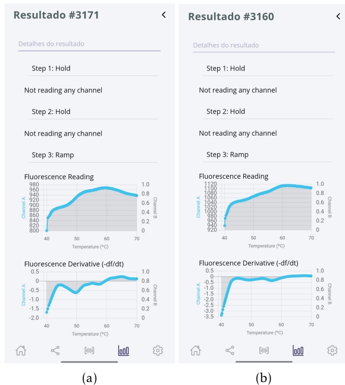
Figure 6.11: Application result page: a) Ramp analysis with an incorrect CC result when it should have been a CT result, b) Ramp analysis with an incorrect TT result when it should have been a CT result.
