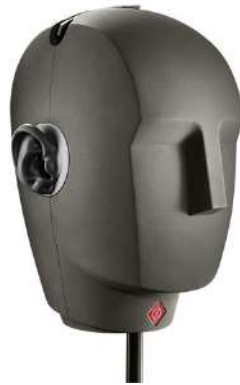
Figure 2.6: Example of a dummy head setup used to record binaural audio [36].
