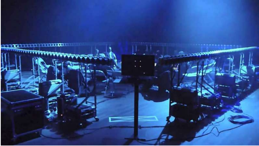
Figure 2.9: Wave Field Synthesis experimental setup with an array of small loudspeakers [23].
