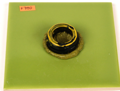
Fig. 16 Glass mouth of a bottle stuck to a glassed tile through some furnace masa with enamel (low).
