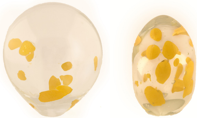
Fig. 26 Blown piece with pieces of masa in the outside and in the inside respectively
