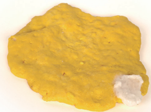
Fig. 25 Borosilicate masa & borosilicate masa with low temperature enamel
