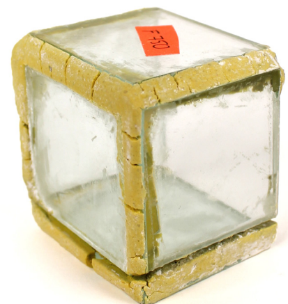
Fig. 15 Window glass sheets joined by window masa with enamel (low)
