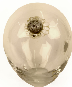
Fig. 35 Blown piece with un-pre-fired masa balls applied on the outside
