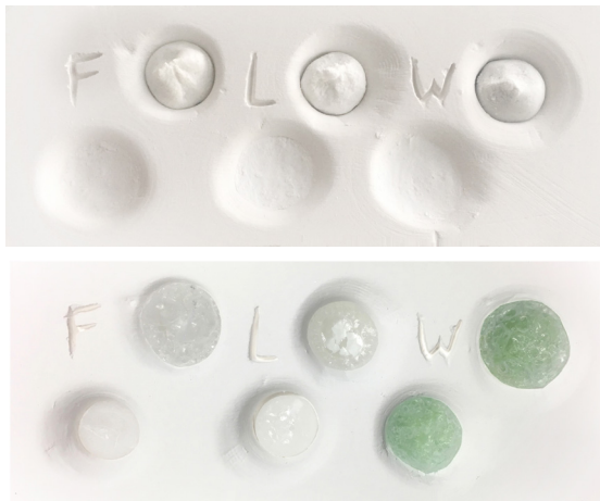
Samples after firing on a plaster and silica mold
