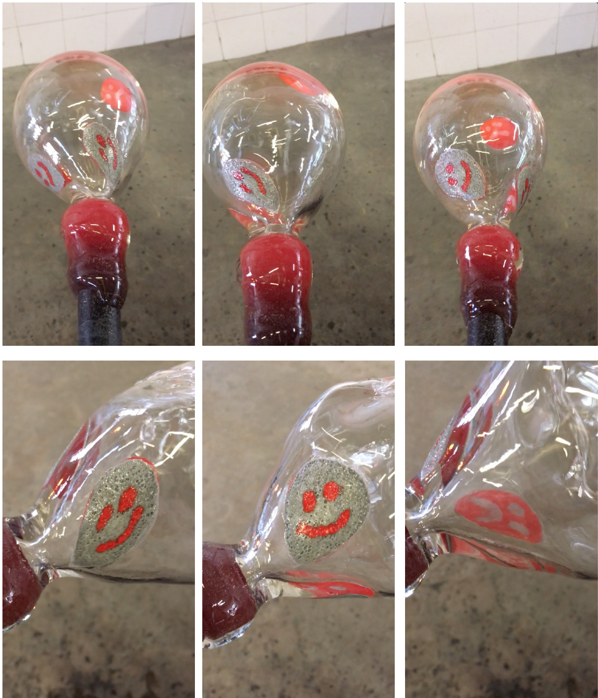
Fig. 30 Blownpiece with the picked masa pieces on while blowing
