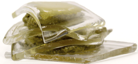
Fig. 13 Furnace glass sheets trapping some furnace masa with enamel (low)
