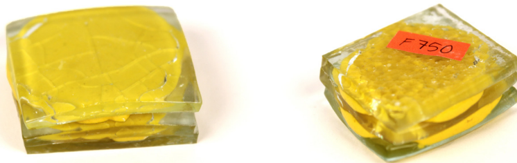
Fig. 12. Window glass sheets trapping some furnace masa with enamel (low)
