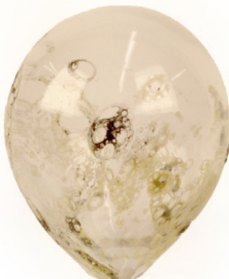
Fig. 34 Blown piece with the remains of un-pre-fired masa applied on the outside
