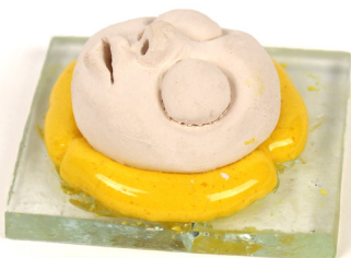
Fig. 14 Window glass sheet and ceramic piece joined by some furnace masa with enamel (low)
