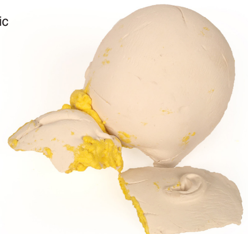
Fig. 23 Ceramic piece & borosilicate masa with low temperature enamel
