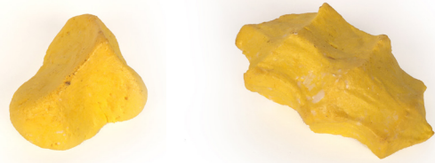
Fig. 24 Borosilicate masa with low temperature enamel
