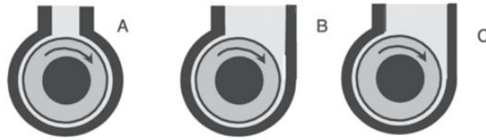
Figure 3.11 Feed pocket configurations [42]
