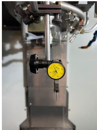
Figure 4.6 Dial gauge with an associated deviation of \Delta = 0.005 mm
