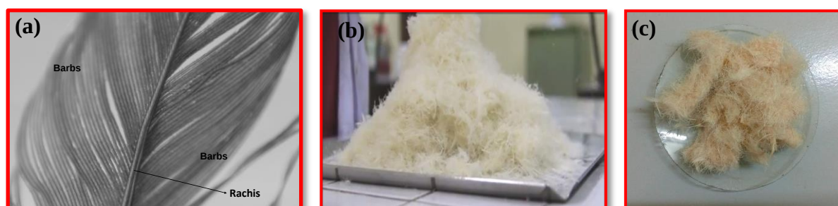
Fig. 1. Chicken feather close-up image showing rachis and barbs (a). Chicken feather barbs before (b) and after (c) modification.
