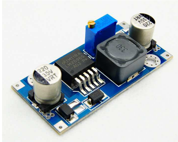
Figura 63 – Conversor DC/DC – LM2595
