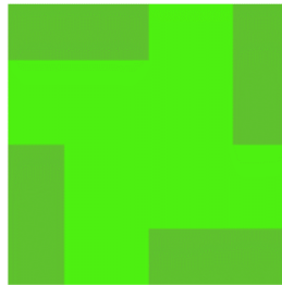
Figure 4.9 – Chiral initial design, with \rho_1 = 0.3 in vivid green elements and \rho_1 = 0.7 in darker green elements, whereas \rho_2 = 0.5 in all elements.
