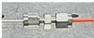
Figure 7.11 - Flow meter attachment to stainless steel capillary tube
