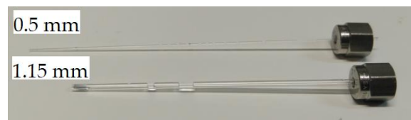
Figure 7.3 - Glass capillary tubes
