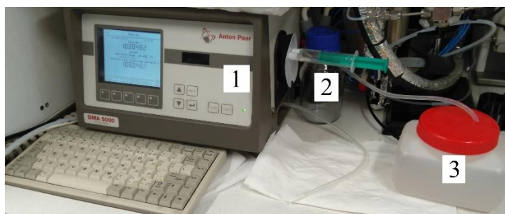
Figure 4.18 – Density measurement experimental setup. Label: (1) oscillation-type density meter DMA 5000 (Anton Paar), (2) BBraun syringe, (3) waste reservoir
