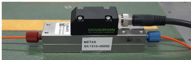
Figure 7.10 - Sensirion flow meter
