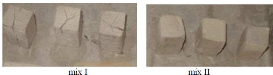
Figure 10– Aspect of specimens subject to salt ageing without linseed oil (mix I) and with linseed oil (mix II)
