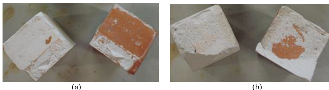
Figure 6 – Illustration of type of failure (a) mix I - adhesive failure, (b) mix II - cohesive failure
