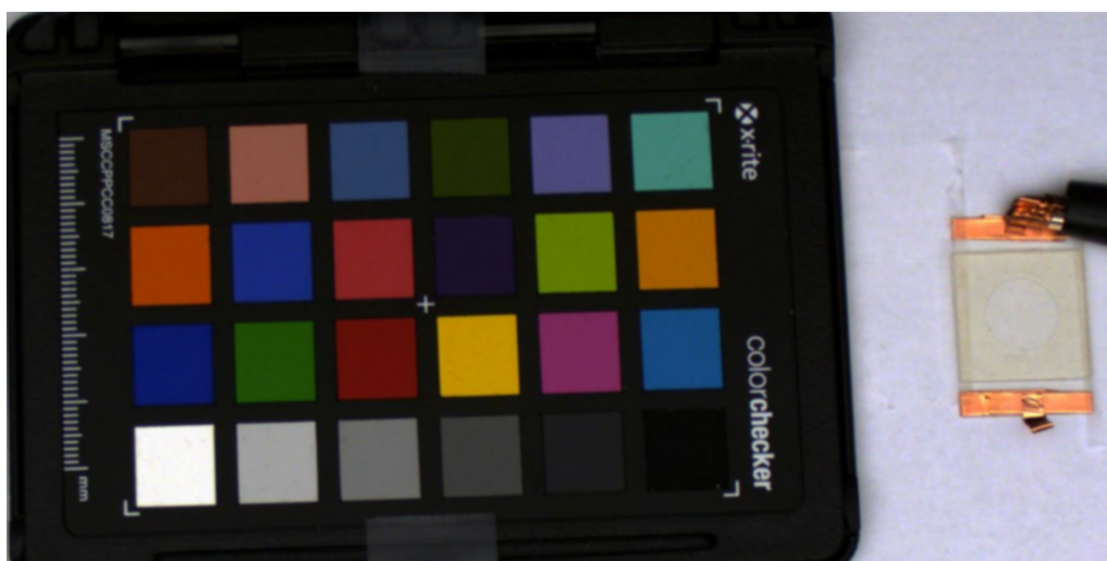
Figure A.1: Digital images of (a) non color corrected, and (b) color corrected irreversible electrochemical indicator with a color checker.
