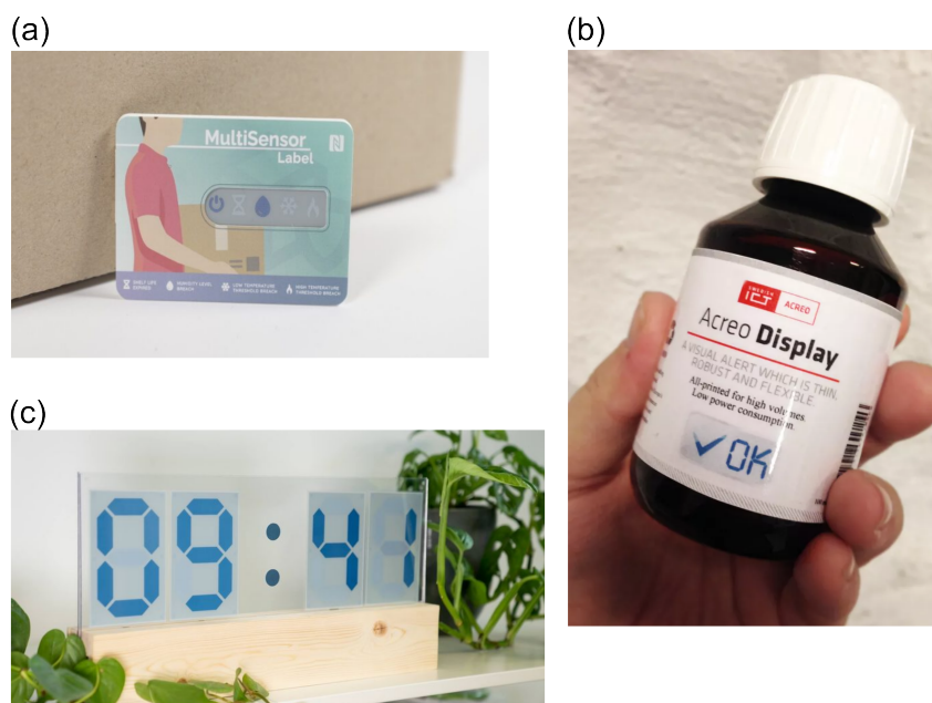
Figure 1.12: Commercial concepts of e-paper type ECDs in the form of (a) a logistics smart label from Ynvisible (b) a flexible pharmaceutical smart label from RISE Research Institutes of Sweden reproduced with permission from ref. [74], and (c) digital signage from Ynvisible.
