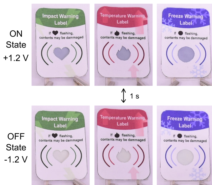
Figure 6.8: Digital images of 2 mC symmetrical indicators with smart label covers demonstrating use cases for impact, high temperature, and freeze warning labels. Indicators are switching with \pm 1.5 V in 0.5 s pulses.
