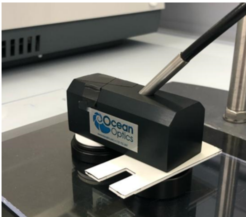
Figure 5.6: Image of optical fiber and probe holder for reflectance measurements. The image is taken while making a blank with the reflectance reference.
