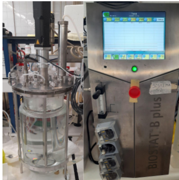
Figure 3.7: Biostat vessel on the left and control tower on the right
