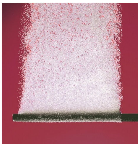
Figure 2.7: Sintered metal sparger example [124]
