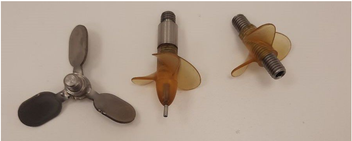
Figure 3.2: Different Impellers used in Stirred Tank Bioreactor system, from right to left, stainless steel elephant ear impeller, bottom marine impeller and middle marine impeller
