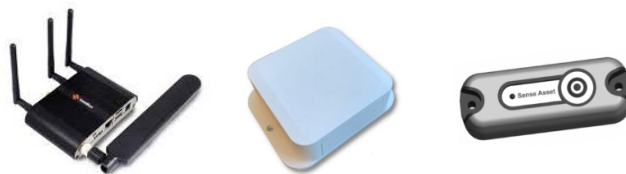
Figure 2.11: Examples of a gateway, anchor, and asset tag respectively, from [43].
