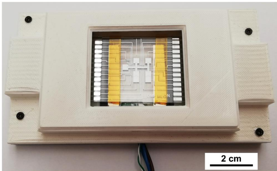
Figure 5.3: a) 3D model of the support system for DMF chips, evidencing all separate components, by fitting order. b) Photograph of the assembled DMF support system, integrated with the DMF device. Note that the top plate of the DMF device was omitted for better visualization.
