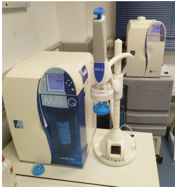
Figure 3-2 Milli Q Advantage water system (Merck Millipore)
