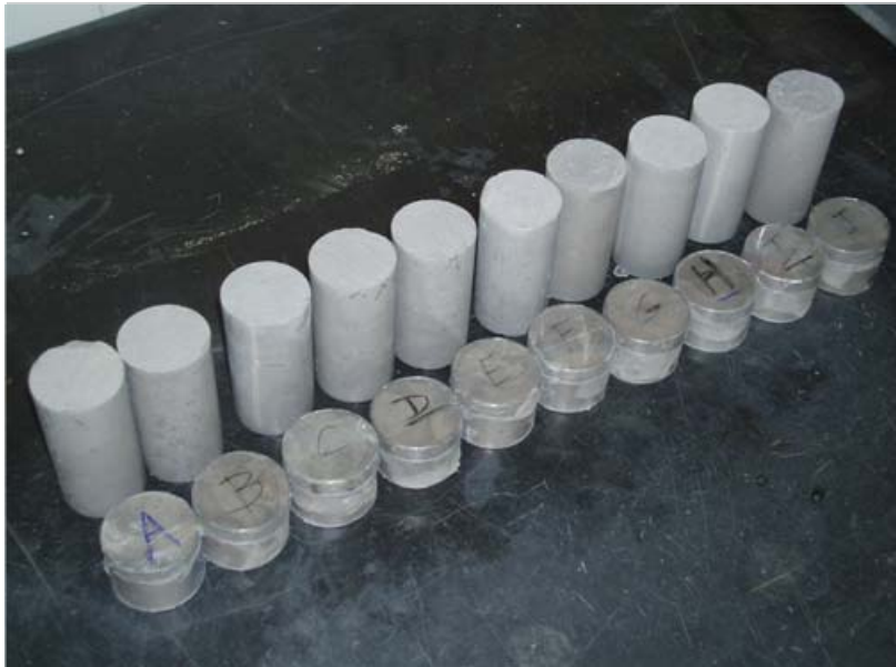
Figure 2.18 - Formulations of the s/s materials prepared with fly ashes
