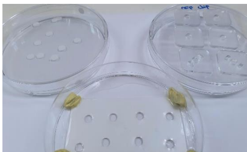
Material needed to assemble the insert layer (PDMS + scaffold + PCR tape with thin layer of PDMS)
