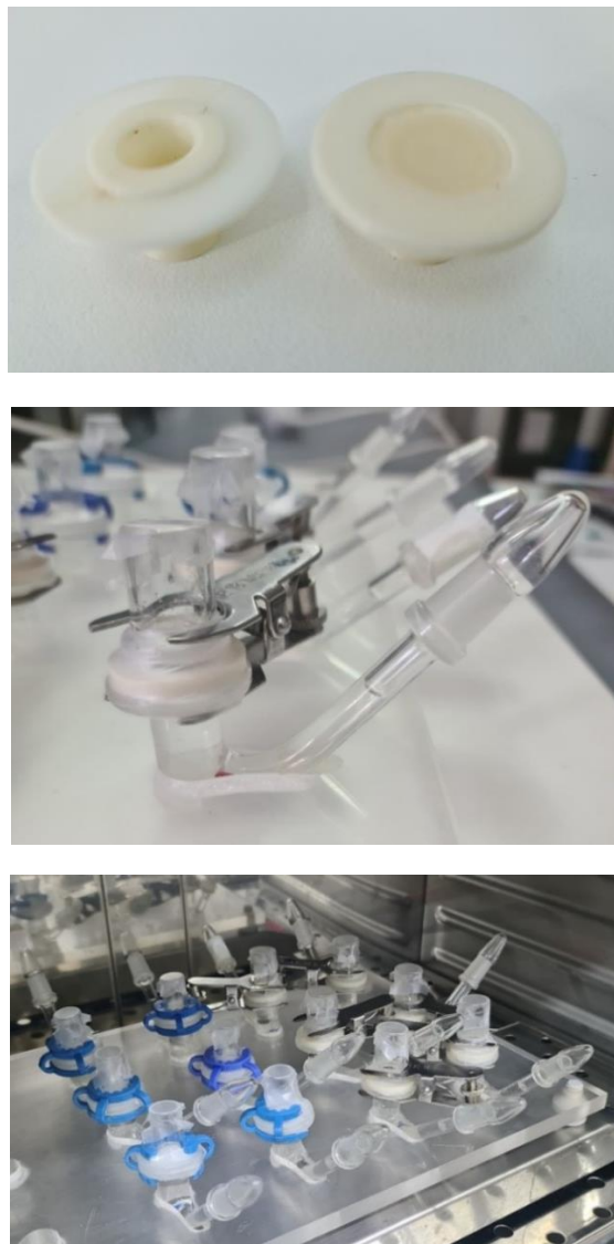
Figure A. 3. Experimental setup of the permeation testing using Franz cells. Top: Photograph of fabricated tailor-made full thickness skin model (FTSm) adapters using 3D printing. The FTSm is lower part has as a small cavity to take up the FTSm. The upper part tightly fixes the margin of the skin model while leaving open an exposure area of 9 mm in diameter. The design facilitates dermal absorption assays under standardized conditions. Dimensions are in mm. Different views: isometric, top and front.
