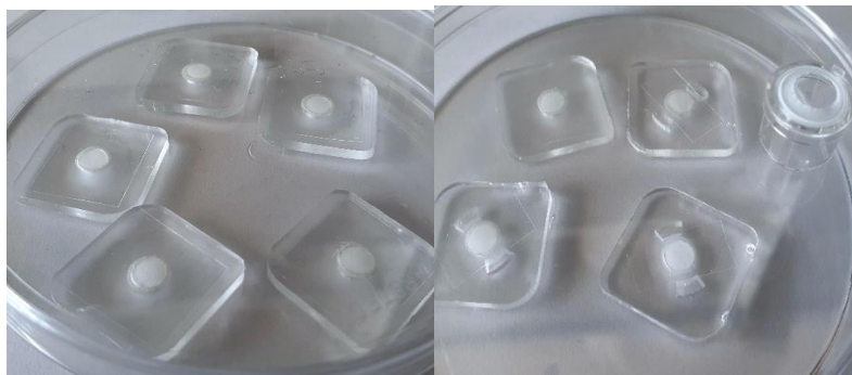
Insert layer with PDMS layer + membrane/scaffold + PCR tape. Left: Insert layer with Alvetex. Right: insert layer with polycarbonate membranes
