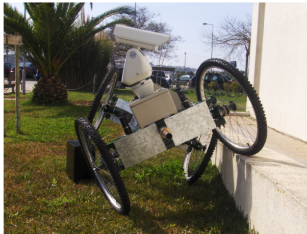
Figure 5.3: Torsion caused by the spinal axle.
